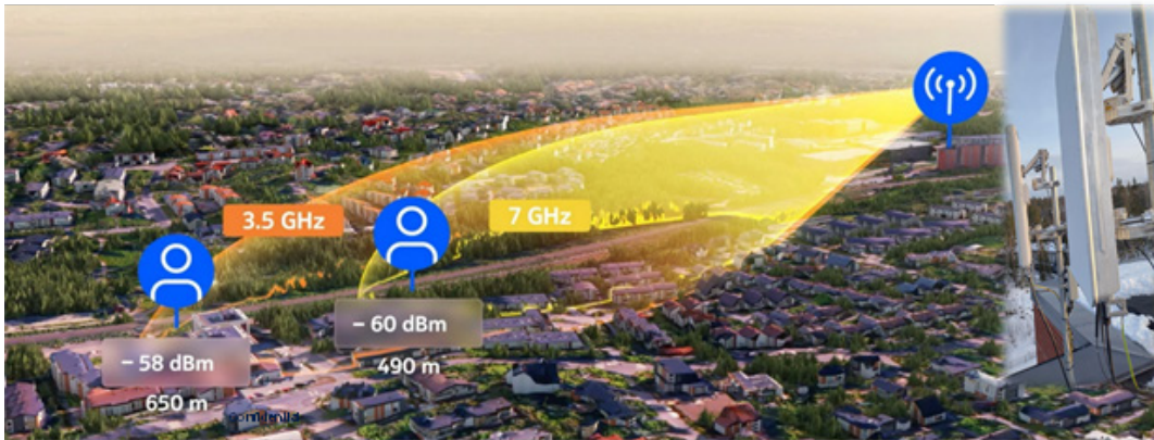
Figure 9: Field measurements in Finland with 7 GHz antenna using 768AE ((Source: 5G Americas member company).
