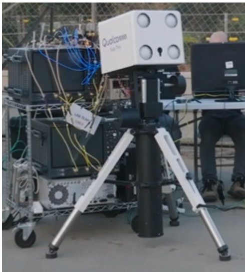
Figure 6: Lens antenna prototype solution capable of delivery 300 Gbps with 100 us latency
