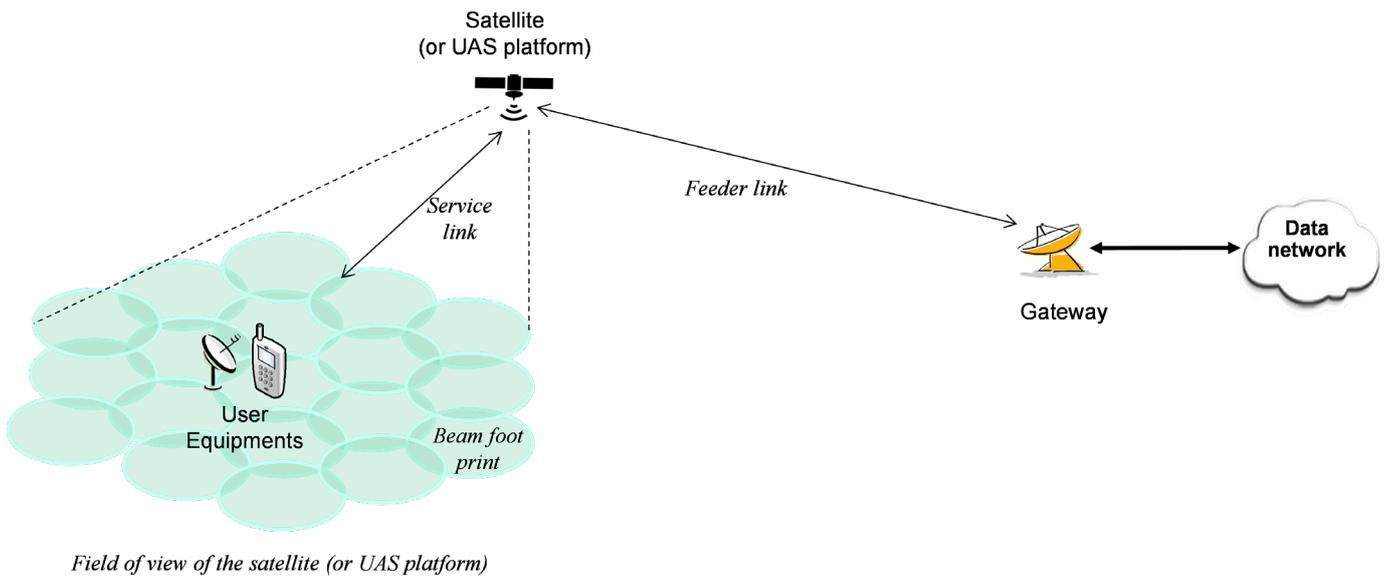
Figure 4.1-3 Satellite-based NTN typical scenario based on regenerative payload (source: 3GPP TR 38.821-g00)
