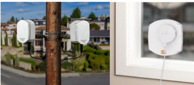
Fig. 5.6. Examples of outdoor (left) and indoor (right) mmWave repeaters.
