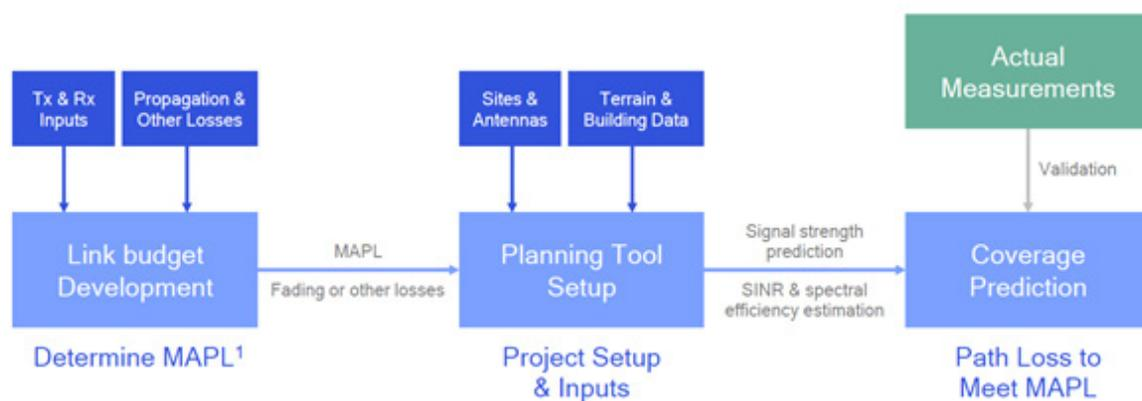
Using the coverage prediction methodology illustrated in Fig. 8.1, the network coverage simulation studies were conducted for a number of cities, including San Francisco. Fig. 8.2 shows a signal strength heatmap for San Francisco based on these 5G NR mmWave coverage simulation results.
