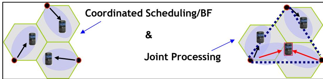
Release 11 also implements CoMP on the uplink, by which multiple base stations receive uplink transmissions and jointly process the signal, resulting in significant interference cancellation and improvements to spectral efficiency.
