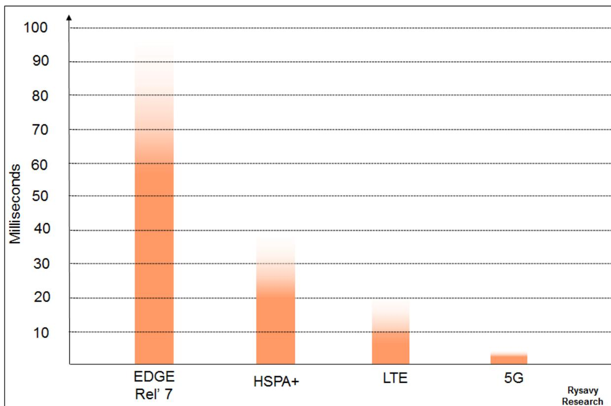
The values shown in Figure 36 reflect measurements of commercially deployed technologies, with EDGE Release 7 achieving 70 to 95 msec, HSPA+ 25 to 30 msec, and LTE 15 to 20 msec. A goal for 5G is less than 1 msec latency.
