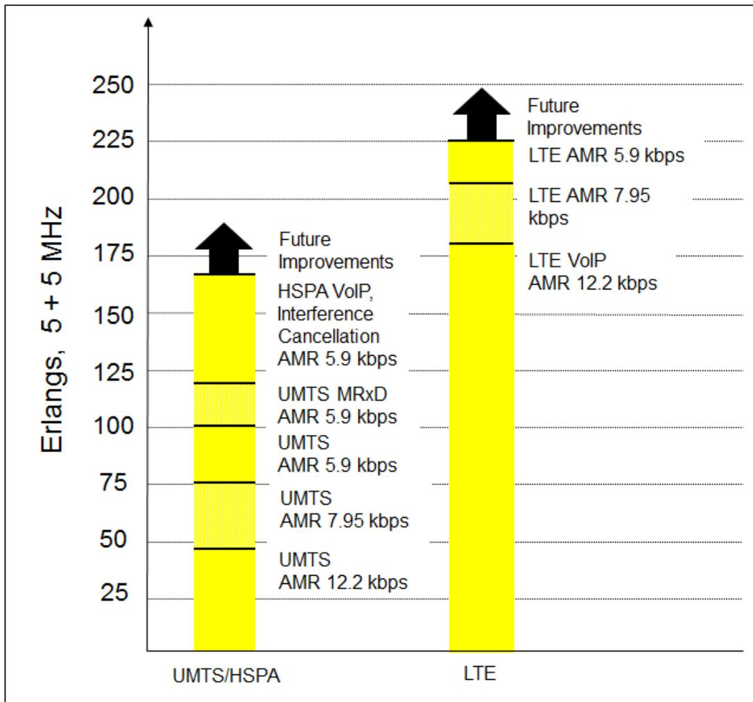
Figure 40 shows UMTS Release 99 with AMR 12.2 Kbps, 7.95 Kbps, and 5.9 Kbps vocoders. The AMR 12.2 Kbps vocoder provides superior voice quality in good (for example, static and indoor) channel conditions.
