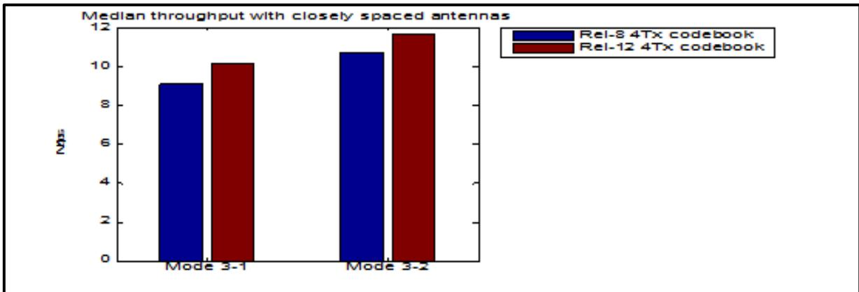
**Figure 48: Cell-Edge Throughput of Feedback Mode 3-2 and New Codebook<sup>119</sup>**
