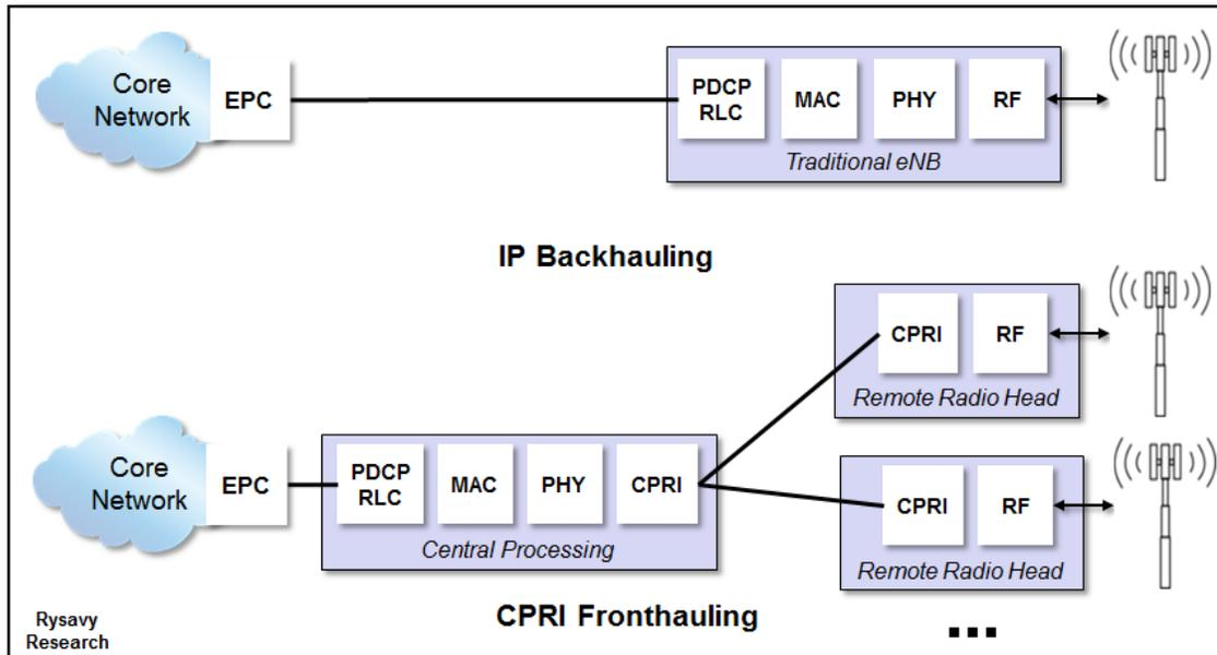
The next evolutionary step after centralizing baseband processing is to virtualize the processing by implementing the functions in software on commodity computing platforms, thus abstracting the functions from any specific hardware implementation.
