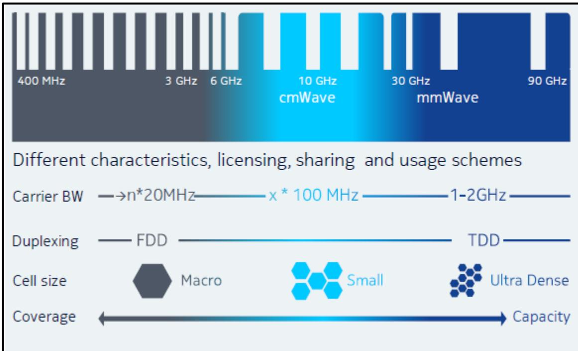
One decision of 5G is whether to use LTE-like radio access in new 5G bands or to instead invent dramatically new radio-access technologies, as shown in Figure 14. New radio
