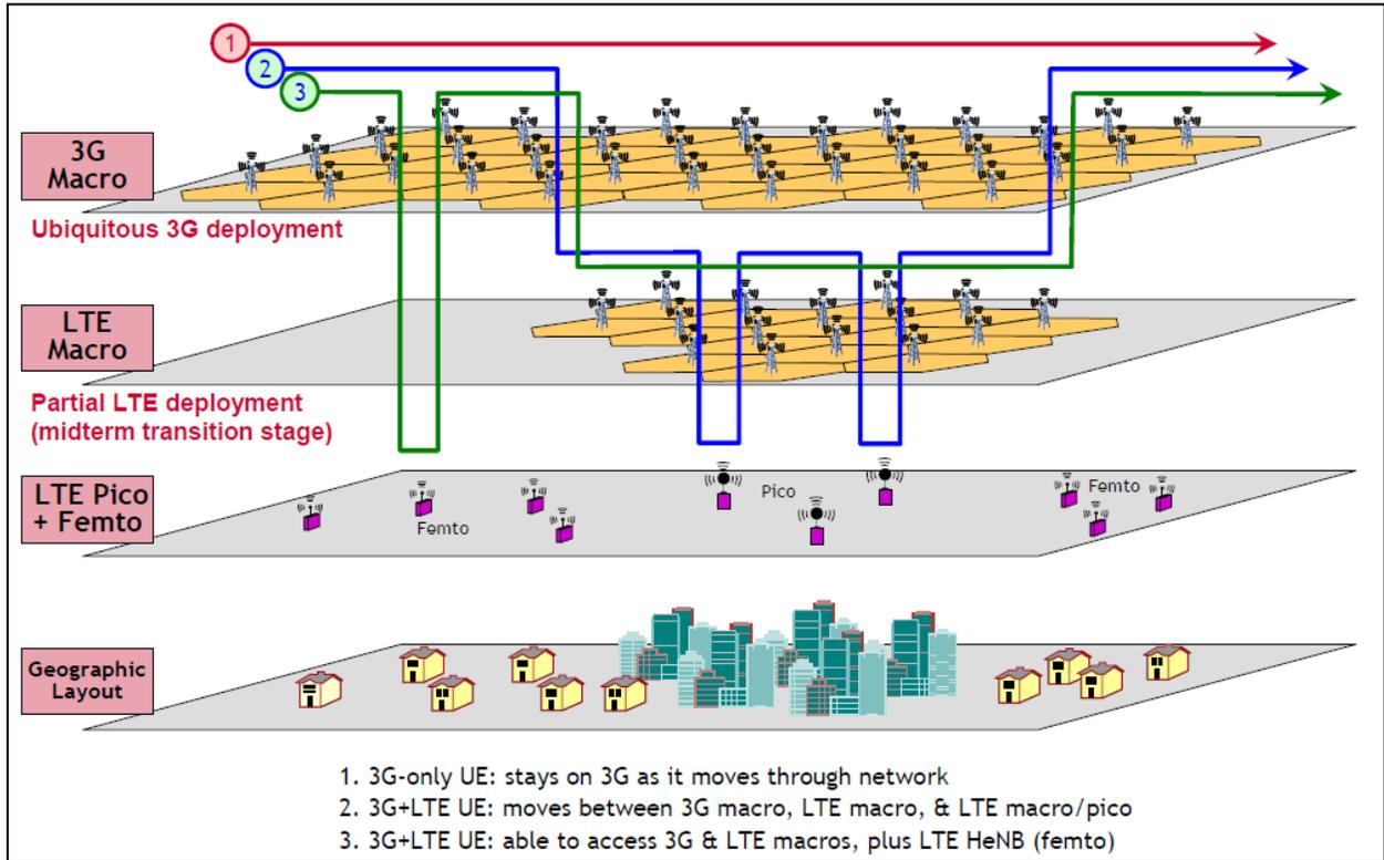
HetNets will allow significant capacity expansion in configurations in which operators can add picocells to coverage areas served by macrocells, particularly if there are hot spots with higher user densities.
