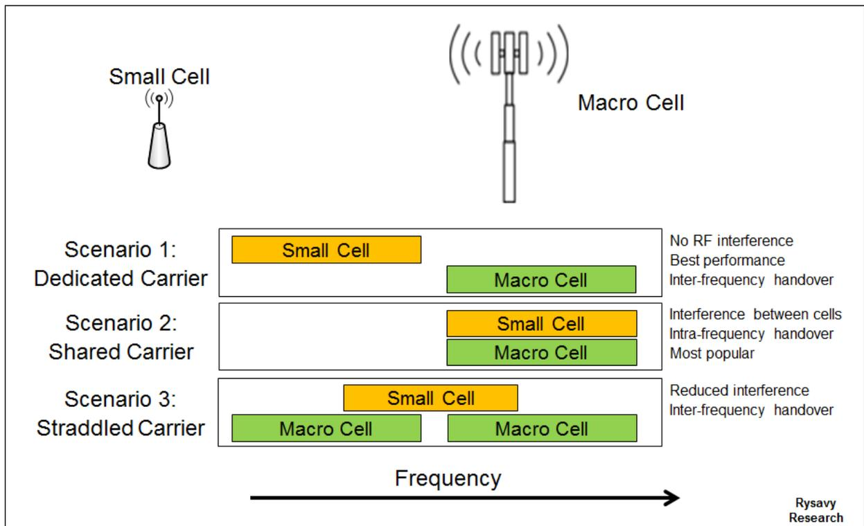
In Scenario 3, the small cells use a straddled radio carrier, accommodating operators with more spectrum, but the network still needs to manage interference using techniques discussed below. Compared with a shared carrier configuration, this configuration has benefits similar to dedicated carriers in terms of radio-parameter planning and reduced interference.
