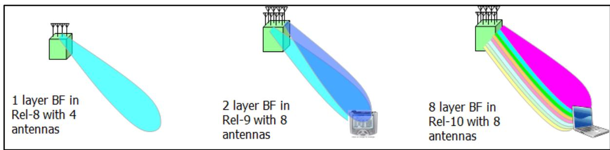
Figure 46 shows multi-user MIMO options across different releases. Release 8 supports two simultaneous users, each with one layer using four antennas, while Releases 9 and 10 support four simultaneous users, each with one layer.
