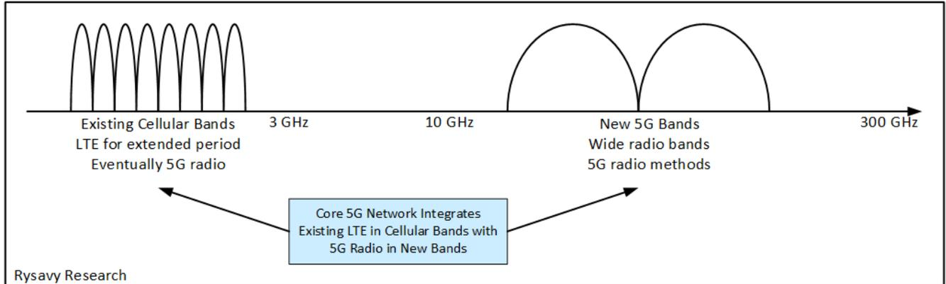
As shown in Figure 13, higher-frequency bands in 5G will provide capacity with smaller cells, and lower bands will provide coverage with larger cells. This is similar to the approach taken in 4G.
