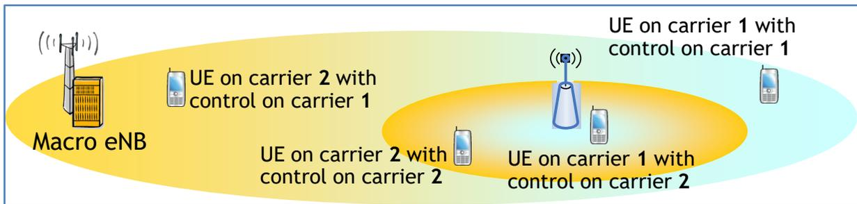
CC1 is the primary component carrier for the macro cell, while CC2 is the primary for the picocell; hence the protected carriers are CC1 for the macro cell and CC2 for the picocell. The macro cell allocates a lower transmission power for its secondary CC in order to reduce
