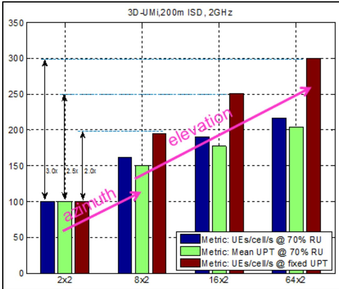
This figure compares 8X2, 16X2, and 64X2 MIMO performance relative to 2X2 MIMO (normalized to value 100). The blue bars (case 1) show the supported number of users per sector (referred to as "cell" in the figure) at a fixed resource utilization (RU) of 70%; the
