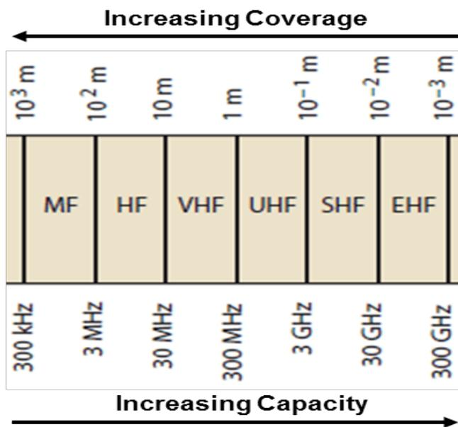
**Figure 1–2** The 5G dense HetNet must embrace a wide range of spectrum bands to achieve the best balance of coverage and capacity
